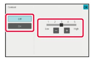
3. Use button or slider to make adjustment. Press OK or START to start scanning.
