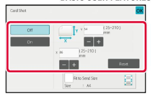
3. Select button ON to enable card shot feature. The size is automatically configured. If you need to scan or print different sizes of card, you can manually change the size.
